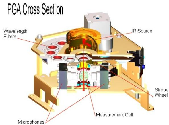
Figure 2. Photo-Acoustic Spectrometer Module.
