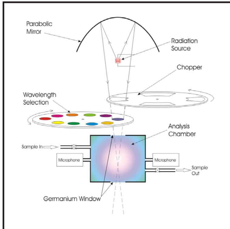
Figure 1. Photo-Acoustic Spectrometer Concept.
