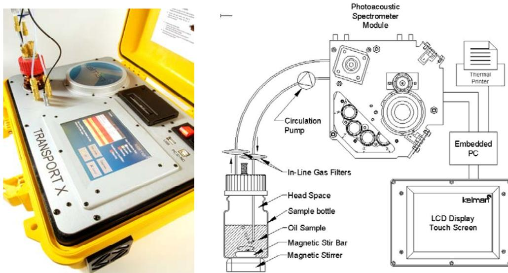
Figure 3. **Transport X** Portable DGA system, Principle of Operation.
