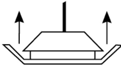
**Shielded light fixtures** use diffusers, lenses and louvers to cover bulbs from direct view; therefore, helping to prevent glare and distribute light.
