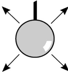
**Indirect light fixtures** distribute 90 to 100 percent of the light upward. The ceiling and upper walls must be clean and highly reflective to allow the light to reach the work area. They provide the most even illumination of all the types of fixtures and the least direct glare. Indirect light fixtures are usually used in offices.
