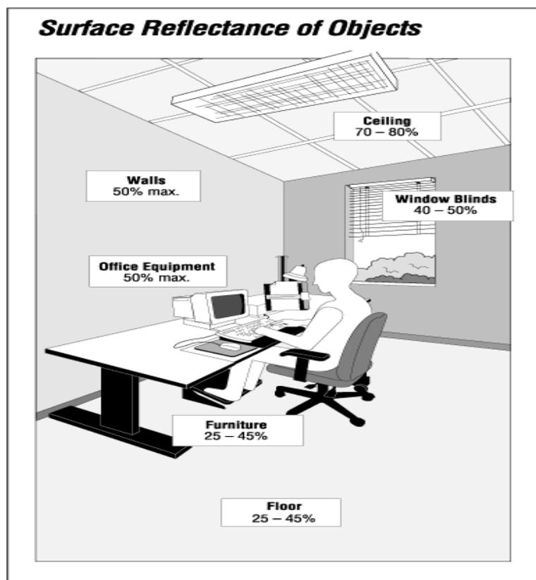
In addition, light fixtures that are too widely spaced or wrongly positioned can create shadows. Objects between the light fixture and work being done can block the light and cast shadows. Likewise, workers sitting with their backs to windows, with light fixtures directly overhead or to the rear, cast shadows on their own work surfaces.
