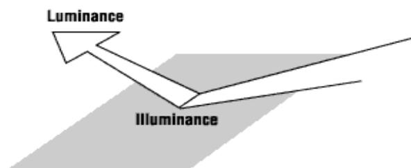
To determine reflectance, the light meter probe is placed on the test surface to measure light falling on the surface. Next, place the probe 5-7 cm away facing the surface to measure the light reflected from the surface. The following formula is used to calculate reflectance:
